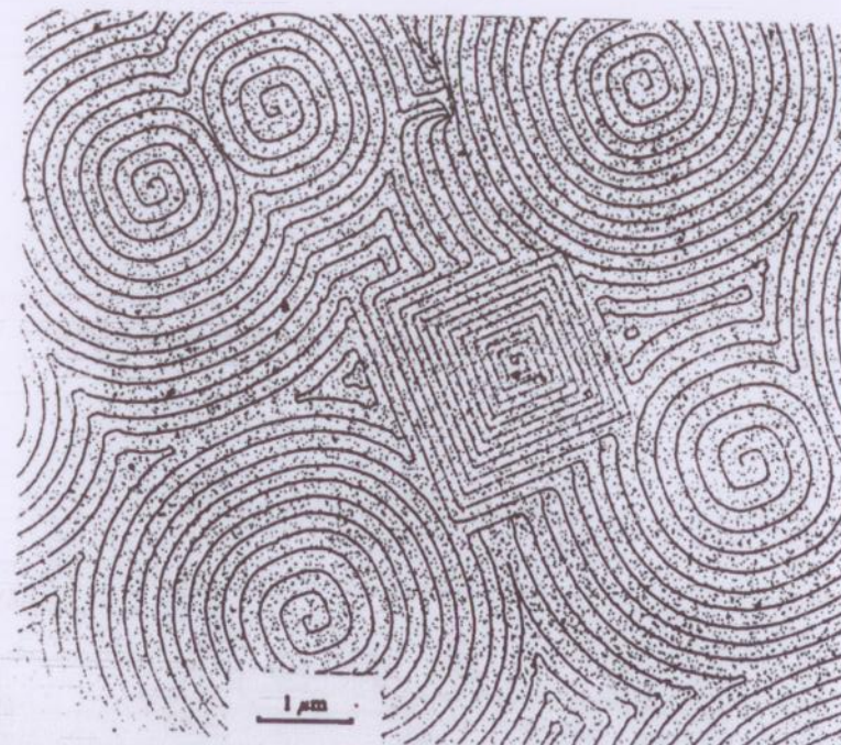
Figure 4.6. Growth step patterns on a sodium chloride cleavage surface revealed by the gold decoration technique (evaporation and preferential adsorption of gold atoms to the ledges on the surface) in a transmission electron microscope. From [10,34] reprinted with the permission of Cambridge University Press.
